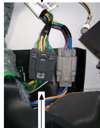
PIN 17 ORANGE/YELLOW WIRE PWM PETROL PUMP SIGNAL CONNECT WITH THE YELLOW WIRE OF EMULATOR
