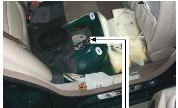
PETROL PUMP ECU LOCATED BELOW THE REAR SEAT PASSENGER SIDE
