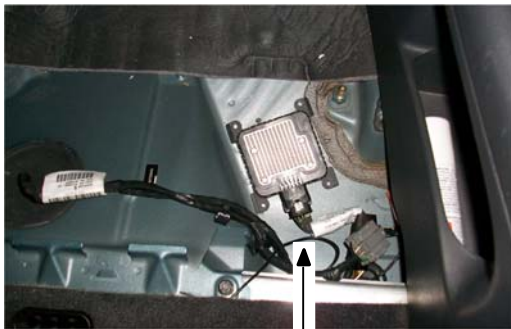
PUMP CONTROL UNIT (located under the seats rear driver side)
